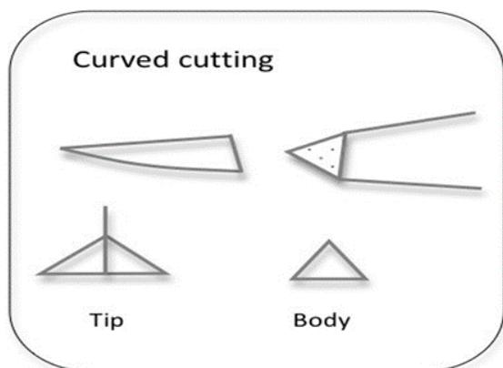
Figure 7: Needle tips - curved cutting.
