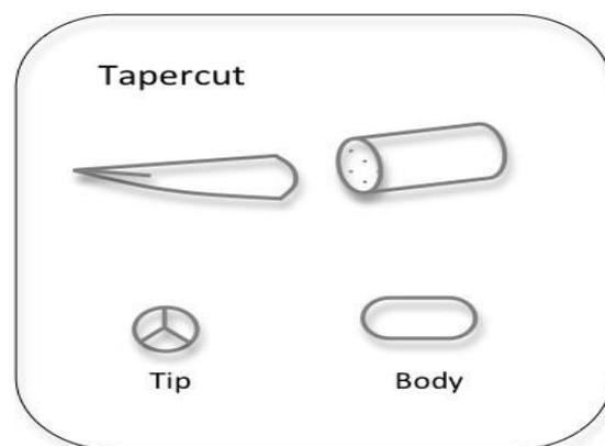
Figure 6: Needle tips -tapercut.
